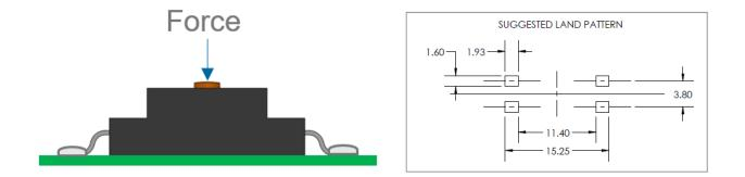
NOTE: Clamping force to the housing may shift the zero reading slightly. Re-zero if needed.
